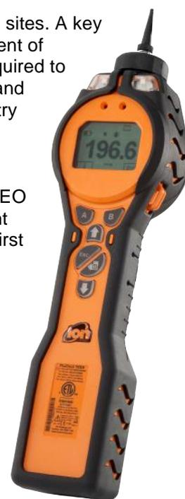
Set points varied from as high as 400 for the HNU PI101 to 260 for the MiniRae 3000, down to 130 for the Ion PhoCheck series, all referenced to Maine's normalised value of 100, with a bigger set point equating to a bigger inaccuracy. Maine DEP and many other users have taken the decision to switch over to the Ion Science PID.
