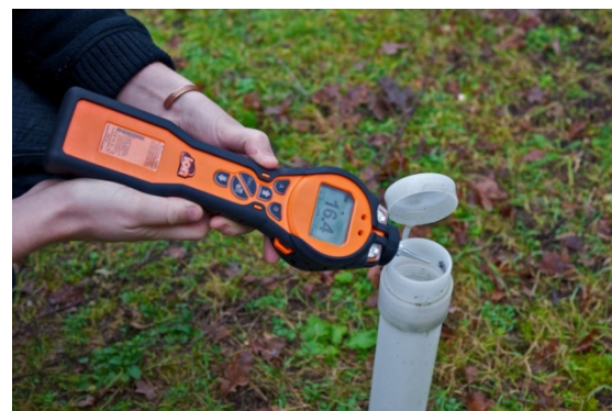
Tiger being used to detect VOCs from contaminated land during headspace analysis
