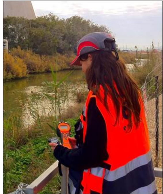
Tiger being used to detect VOCs during dredging of Israel's River Kishon
