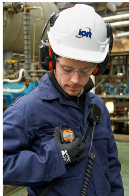
*Cub personal PID monitor used to detect VOCs at refinery.*
