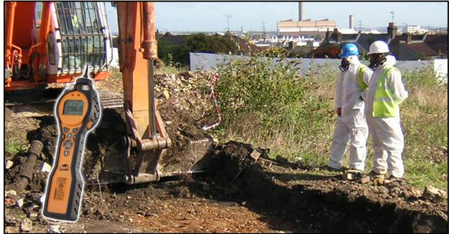
Recommended by Ion Science's exclusive UK distributor, Shawcity Ltd ([www.shawcity.co.uk](http://www.shawcity.co.uk)), as a replacement for equipment that was no longer supported by its manufacturer, the revolutionary Tiger PID (photoionisation detection) instruments enable Southern Testing to make an assessment of risk associated with ground-borne vapour, and also to screen soil samples, which then allows them to make the best use of their laboratory analysis budgets.
