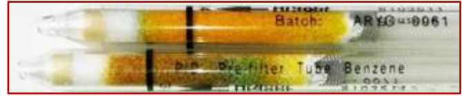
Figure 2. The lower tube has discolouration the \frac{3}{4} mark indicating the tubes capacity may have been reached.
