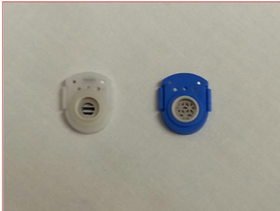
*IonPID* production stack A-846229, left, and the new HPPM stack reference A-846486, right.
