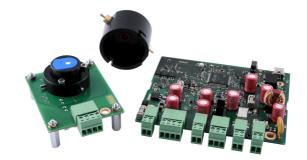
The Sensor PCB acts as a sensor breakout board enabling users to insert a MiniPID photoionisation detection (PID) sensor and perform basic sensor testing. It can also be connected to the Integration PCB to make it really simple to add PID sensors to any application.
